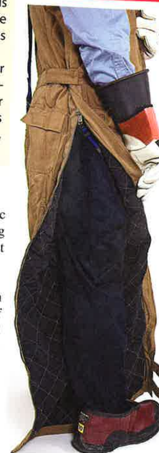
An arc-rated PPE system of clothing. (Courtesy of Salisbury by Honeywell)
