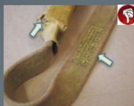
Missing label: damage to protective sleeve over energy absorber
