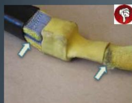
Abrasion damage adjacent to energy absorber: displaced protective sleeve over energy absorber
