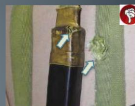
Damaged webbing and protector to energy absorber
