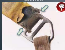
Wear at end of absorber loop at connection
