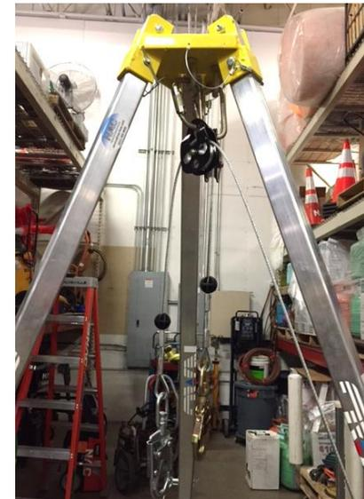
Pulley attached to tripod head
